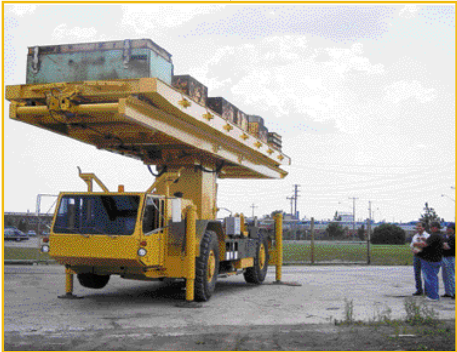
Arva Industries built this roof panel installer to lift and help position heavy ceiling tile for the $10.8 billion "Big Dig" project in Boston. The machine was tested in St. Thomas with a load of 30,300 kilos.
