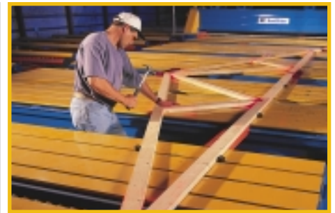
Virtek's templating technology is used by the TrussLine(R) system, which is used in pre-fabricated construction of roof trusses.
