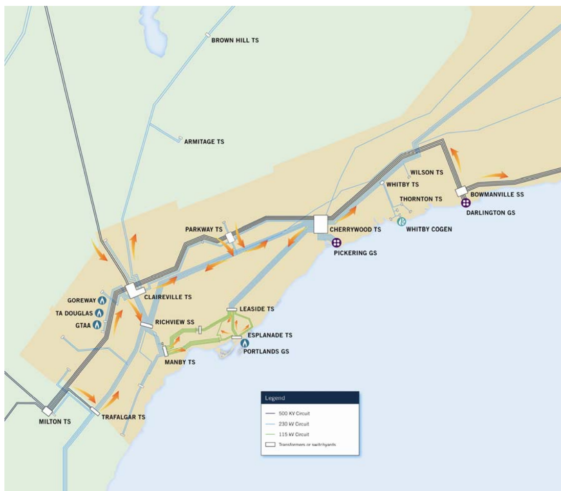
Figure 6.1 Greater Toronto Area Electricity System
