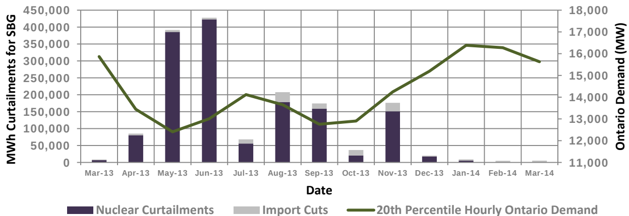
Figure 6.1: MWh Curtailments for SBG versus Ontario Demand
