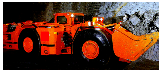
Load-Haul-Dump (LHD) vehicles such as this one are used to move ore in underground mine drifts. Designed for maximum load capacity and for fitting within confined environments, they usually offer very poor operator visibility.
