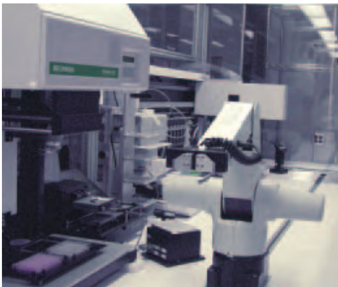
Microarray Robot, paints microscope slides with the DNA of fish. This leading technology enables thousands of genes to be studied at once, making experiments faster to complete.
