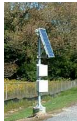
▲ Solar-powered site boundary radiation monitor.
