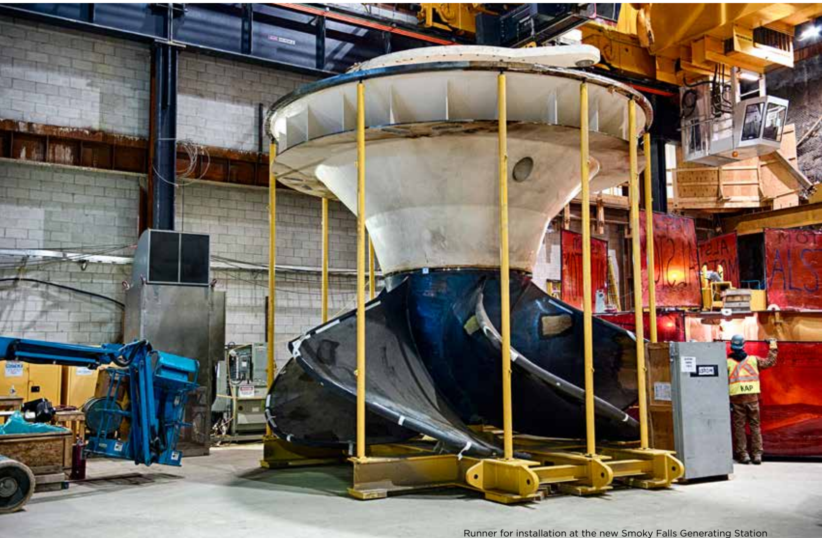
Runner for installation at the new Smoky Falls Generating Station
