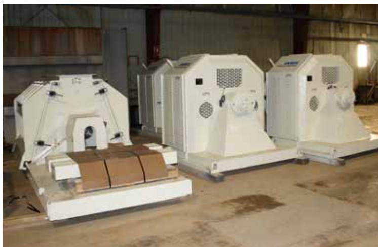
Biomass fuel pellet mills used to produce fuel for Atikokan Generating Station
