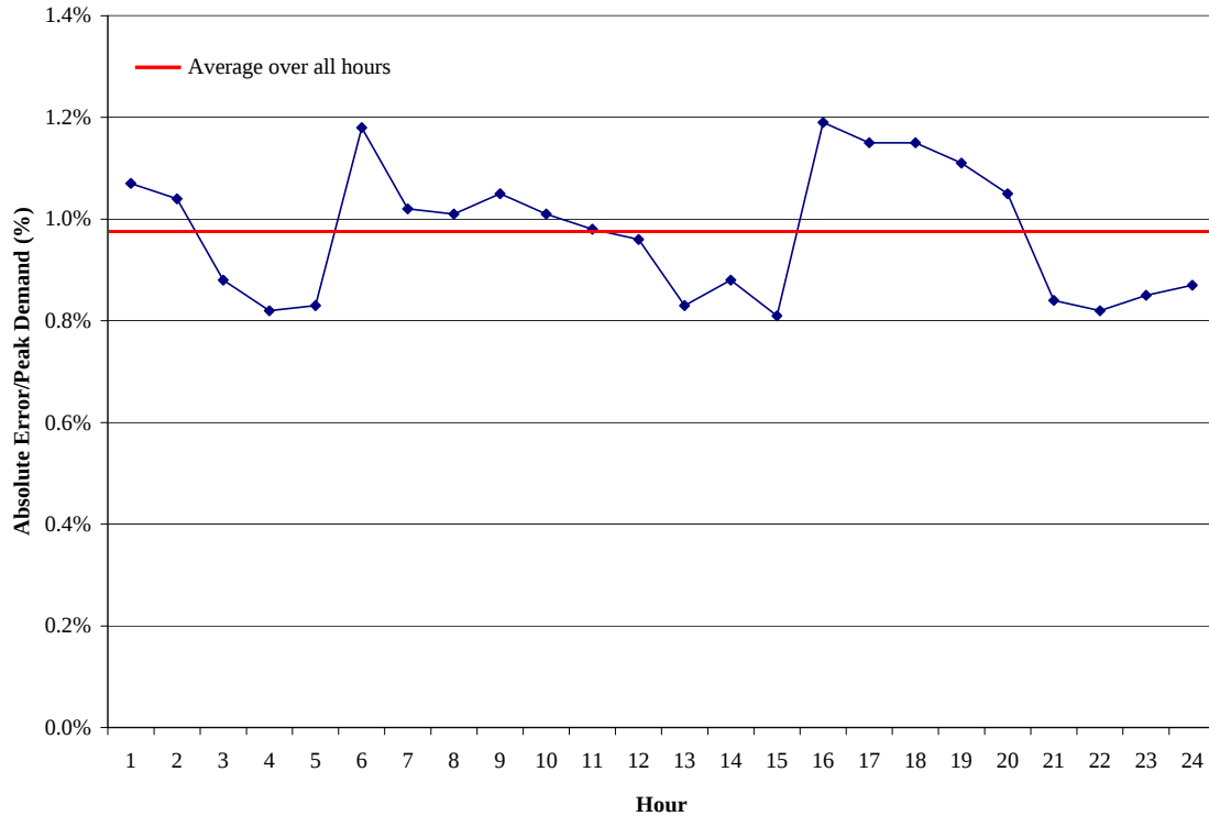
Figure 1-5: Absolute Average One-Hour Ahead Forecast Error by Hour, November 2007 - April 2008 (% of Peak Demand)
