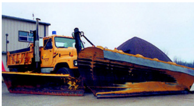
A plough truck complete with the new rubber blade.
