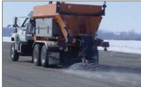
Rear-discharge spreader broadcasting salt across one lane
