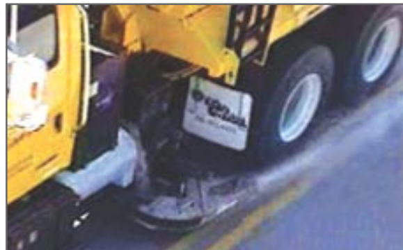
Side-discharge spreader placing salt at centreline
