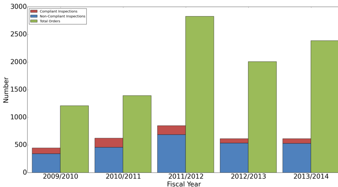
Figure EM-6: Number of orders and compliant and non-compliant periodic inspections conducted on escalators and moving walks over the last five years.
