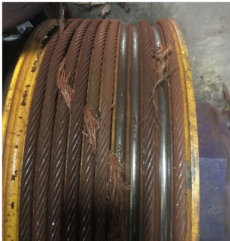
Figure 16: Rough and Frayed Hoist Rope
