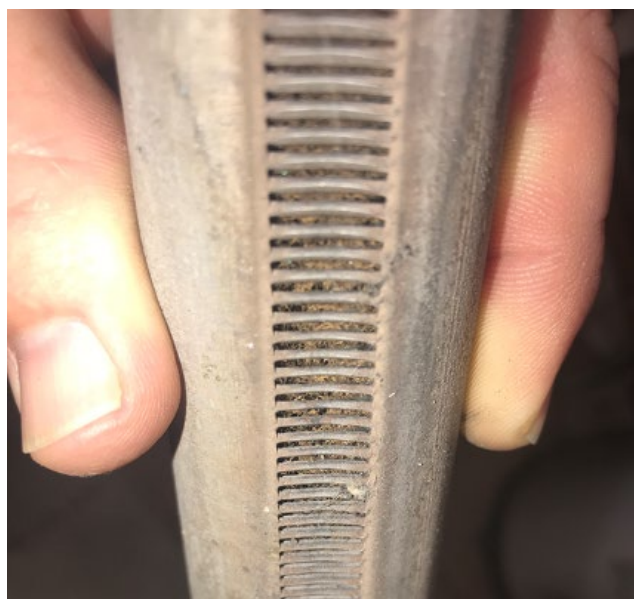
Figure 30: Animal Hair Clogging Burners
