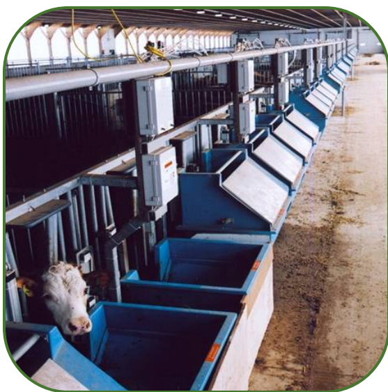
Figure 2. Automated feeding station in Elora Beef Cattle Research Centre, University of Guelph.
