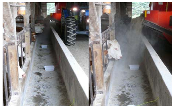
Figure 1. Pans placed in a bunk for sequential analysis of Manganese to determine a mixer CV
