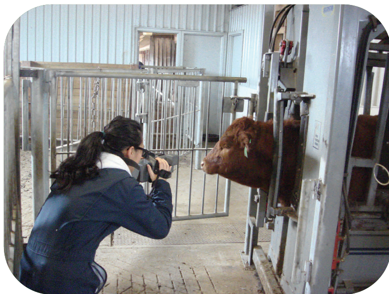
Figure 1 Infrared imaging assessment (head imaging) of a heifer restrained in a squeeze chute.
