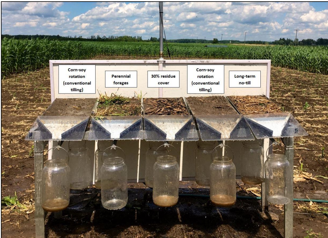
Figure 2: This rainfall simulator shows how soil management decisions affect water infiltration (vials in the background), overland runoff (vials in the foreground), and resulting soil erosion.
