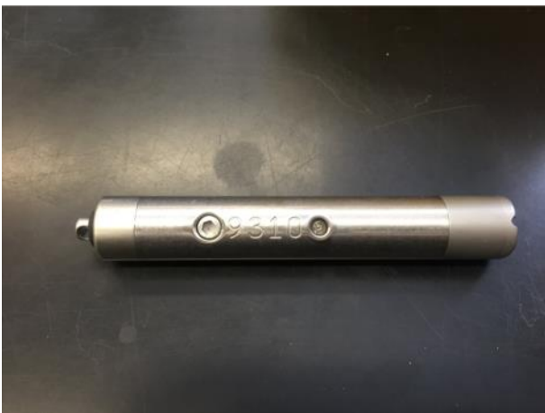
Figure 1 - Reticulo-ruminal pH probe.
