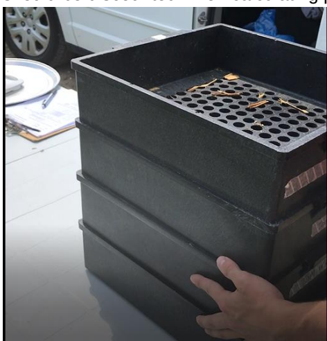
Figure 1 – Penn State Shaker Box used to measure particle size distribution in ruminant rations
