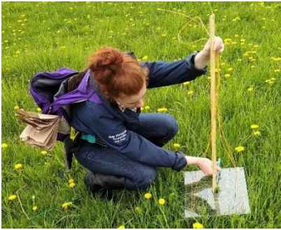
Figure 1. Falling plate meter used to acquire bulk height measurement on pasture
