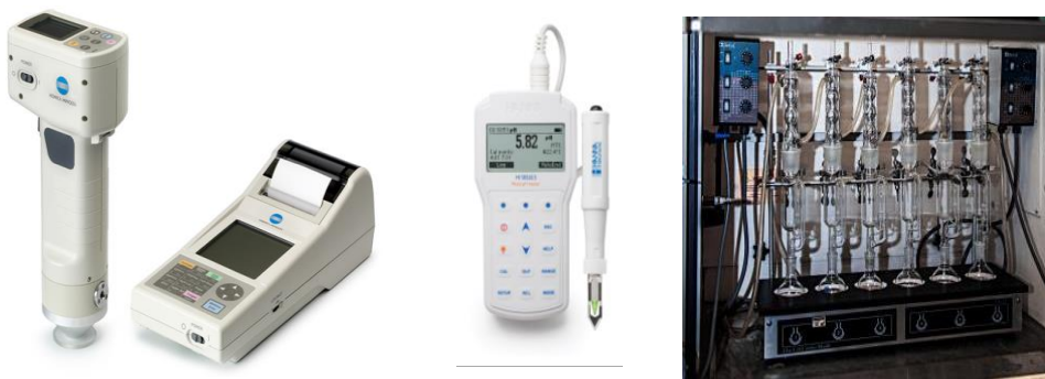
Figure 1. Left to right: Minolta handheld spectrophotometer, pH meter, and Soxhlet extraction apparatus used for determination of extractable intramuscular fat
