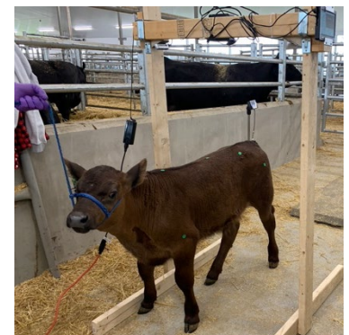
Calf standing under the prototype camera system used to capture visual data to estimate body weight
