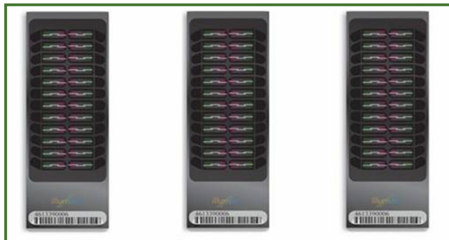
Figure 3. La puce Illumina BovineSNP50 MD Beadchip
