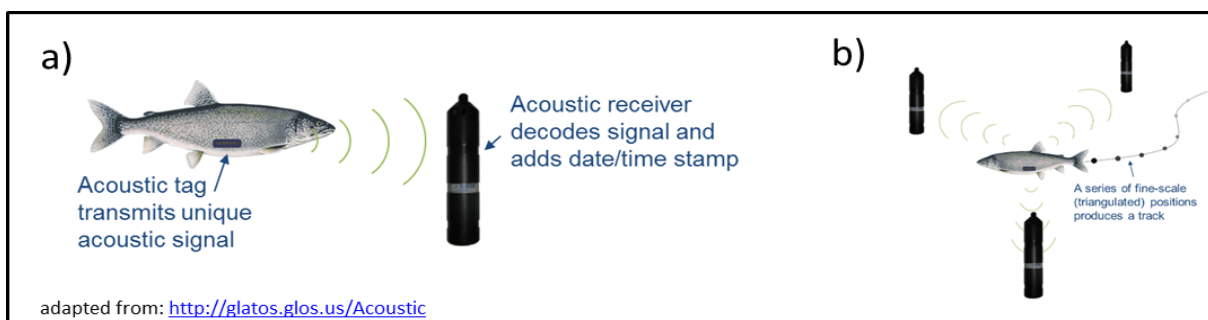
Figure 7.1 How Acoustic telemetry works.
