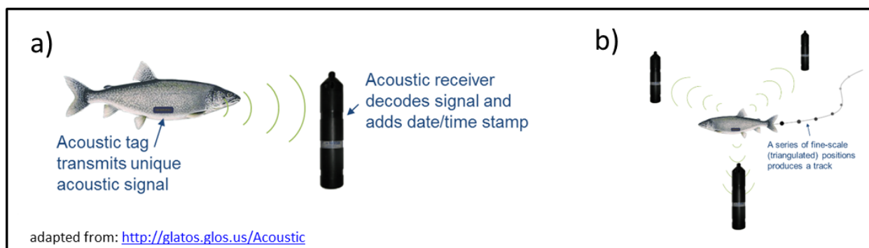
Figure 6.1 How Acoustic telemetry works.
