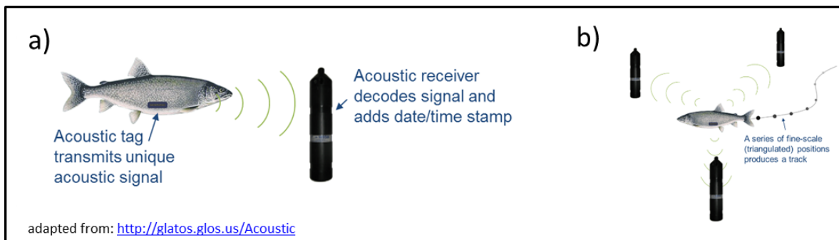
Figure 6.1. How acoustic telemetry works.
