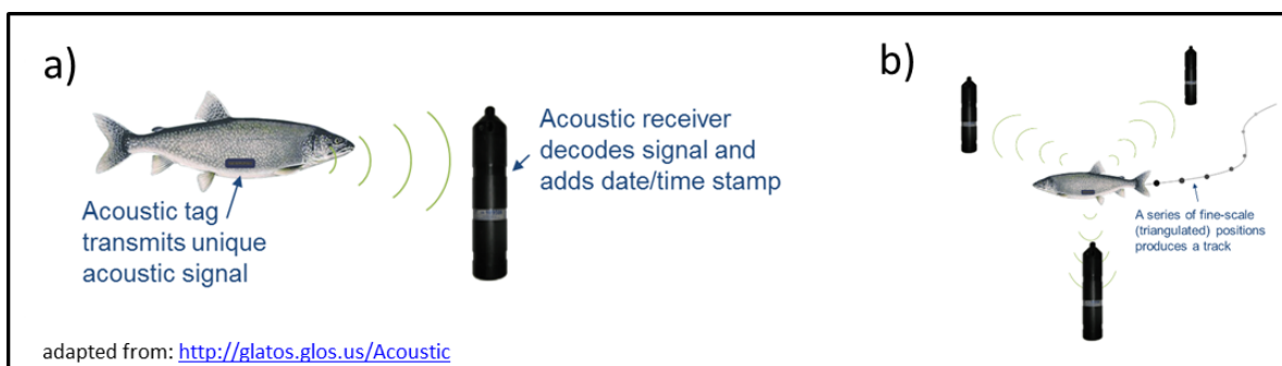
Figure 6.0.1 How acoustic telemetry works.
