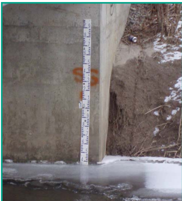
Above: One of 35 staff stream gauges located around the watershed to assess conditions in the event of a flooding emergency.
