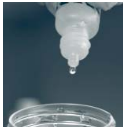
Adding preservative to drinking water sample
