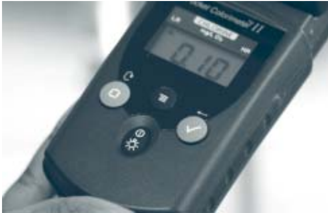
Hand-held chlorine residual analyzer
