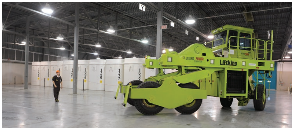
Dry Storage Container transport vehicle at Pickering Waste Management Facility
