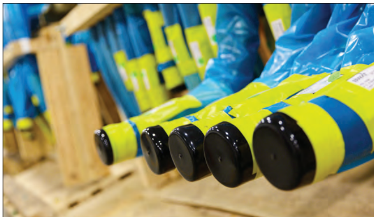
Feeder tubes being prepared for shipment to Darlington Nuclear Generating Station where they will be installed in the Unit 2 reactor.
