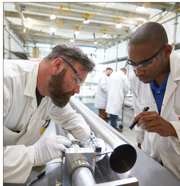
Calandria tubes being inspected at the Darlington Energy Complex.
