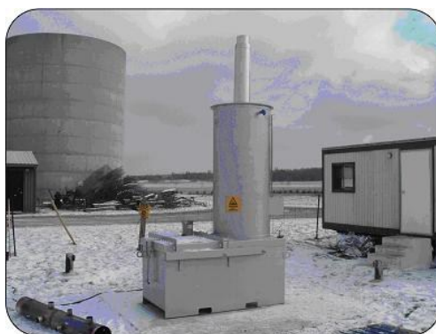
Figure 3: (from left to right) three-bin composting system; Incinerator with a secondary chamber; digging a burial pit using a backhoe
