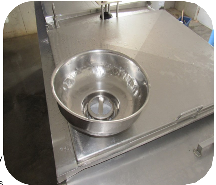
Figure 3: A milk strainer with a properly secured filter disc.
