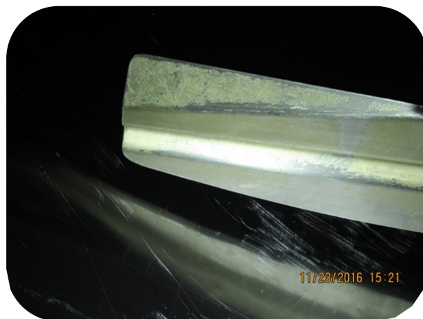
Figure 2: Agitator paddle with a milk fat build-up.
