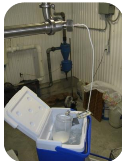
Figure 11 – Group sampling using a QMI sampling elbow. Every time the milk pumps from the receiver jar, a stream of milk can be collected into a sample container.
