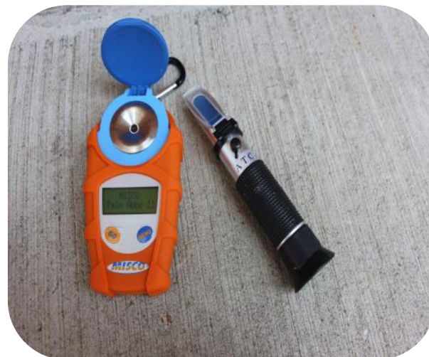
Figure 14. An example of a digital refractometer (left), and a temperature-corrected optical refractometer (right).
