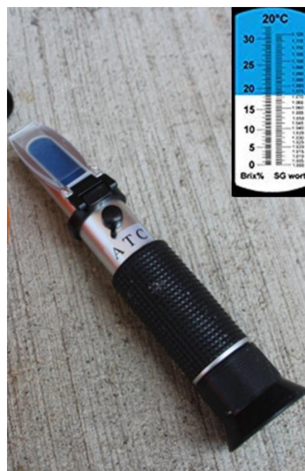
AN OPTICAL REFRACTOMETER AND AN EXAMPLE OF A READING TAKEN FROM AN OPTICAL REFRACTOMETER.
