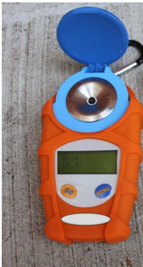
A DIGITAL REFRACTOMETER WITH A PROTECTIVE RUBBER SLEEVE DISPLAYS A READING OF 15.9% BRUX.
