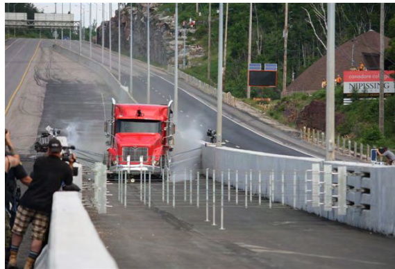
Test truck using the runaway ramp
