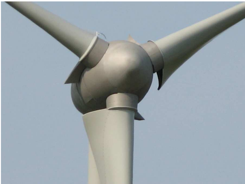
One of the installed ENERCON E82 wind turbines; the turbine has a rated capacity of 2 MW
