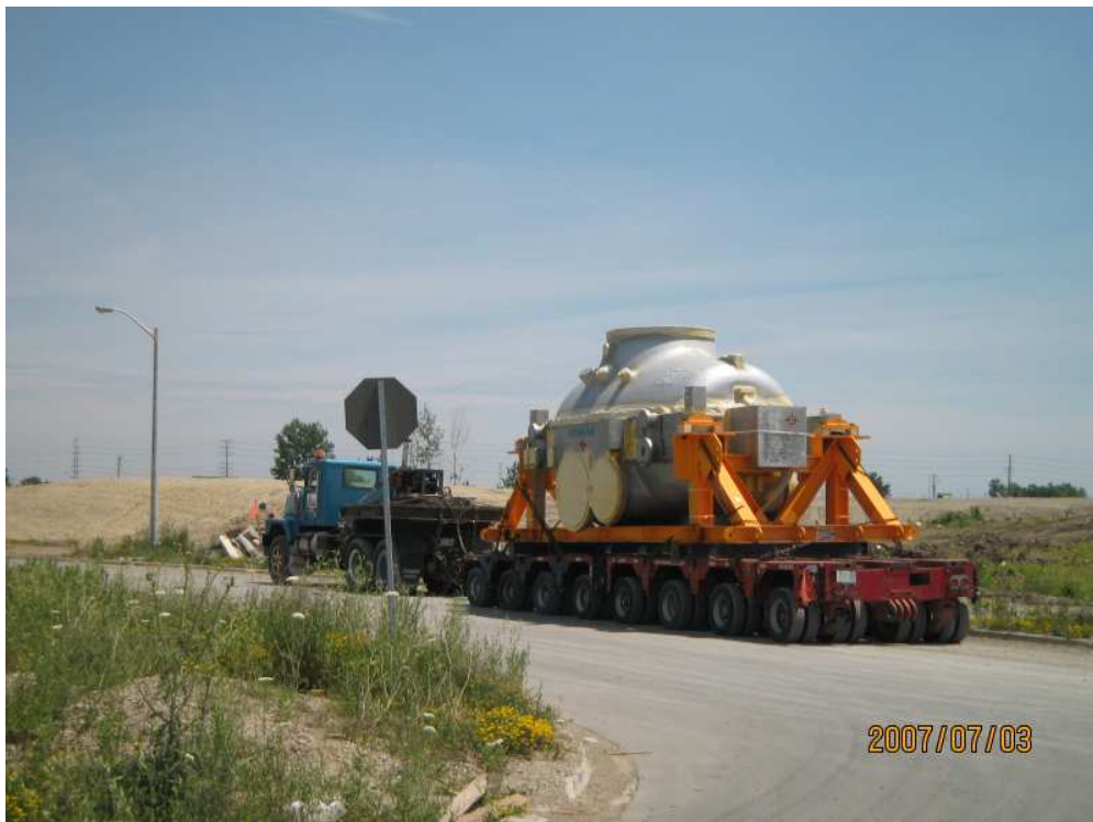
Steam turbine being delivered to the Goreway site
