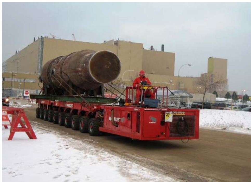
The last of the old steam generators for Unit 1 is being transported to the waste management facility located three km across the Bruce Power site.
