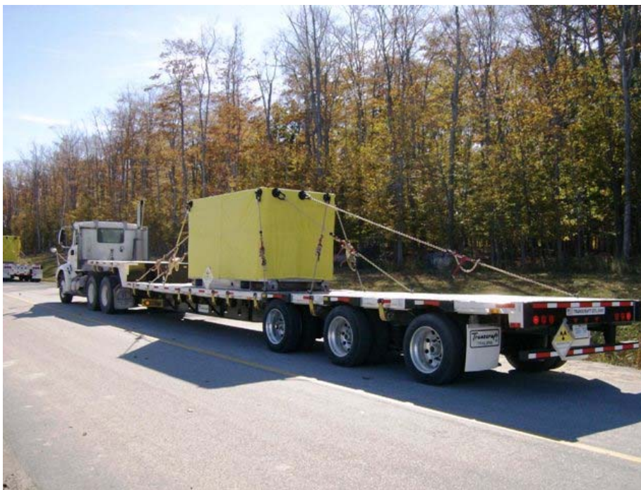
Once filled with used reactor end fittings, the lids are permanently welded to the containers. The containers are then transported to the waste management facility on the Bruce Power site.
