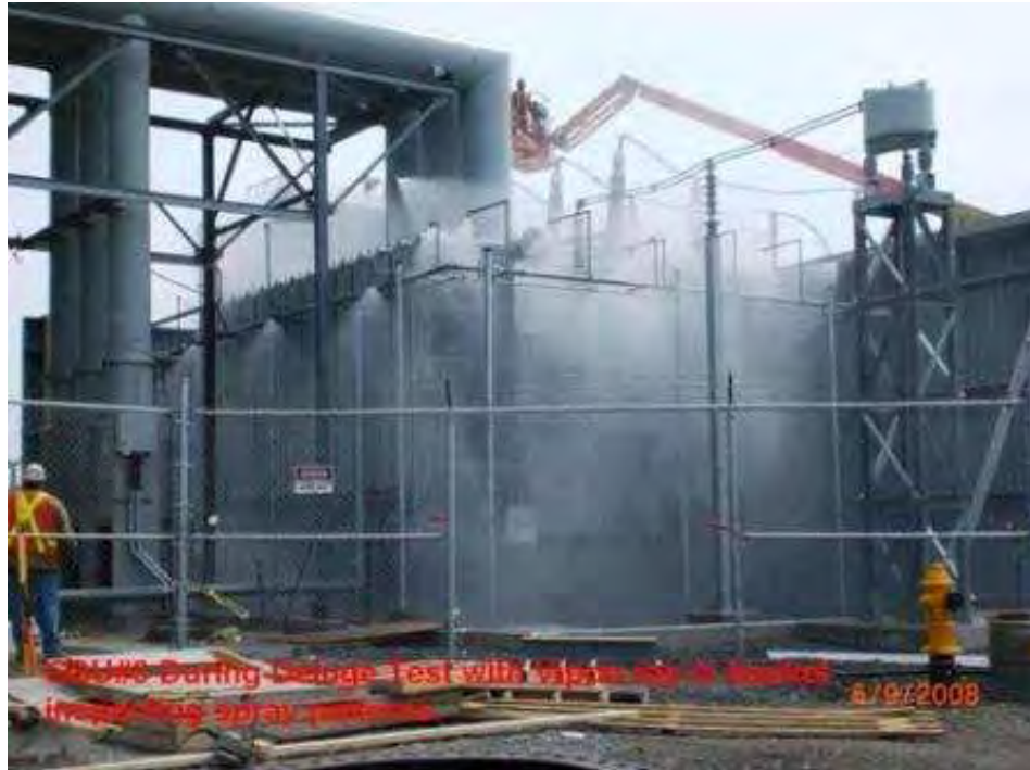
Deluge test being performed at one of the step-up transformers
