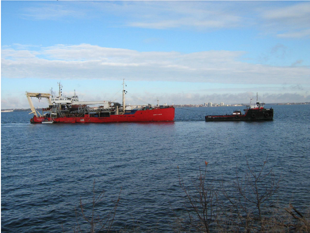
A tugboat positioning a submarine cable-laying vessel for the Wolfe Island Wind Project
