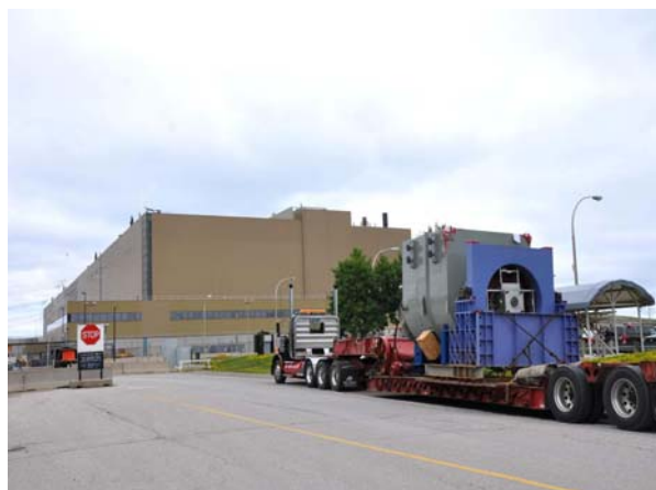
Figure 22 – The program to restore the Primary Heat Transport (PHT) system in unit 2 advanced significantly on July 19 when a rebuilt PHT pump motor returned to the plant. The PHT motor had gone out to Electra Technology Inc. in Hamilton for rebuild, including a rotor rewind, and then to a Westinghouse facility in Pittsburgh for final testing.
