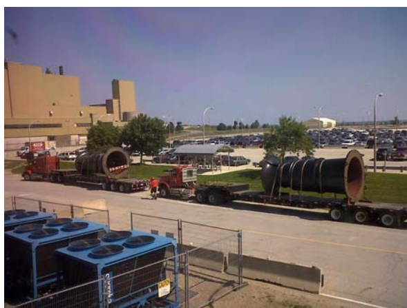
Figure 21 – The refurbished CCW pumps returning to the station on July 29. Each pump is rated at 1.1 MW or 1,450 horsepower, circulating about 776,000 litres of water per minute.
