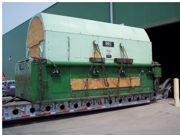
Figure 11 – A view of the generator stator being moved to the storage facility. Inspection of the generator unit is complete and a quote is issued for the refurbishment. Detailed refurbishment engineering for the turbine is in progress. Detailed engineering firm and project manager were selected.
