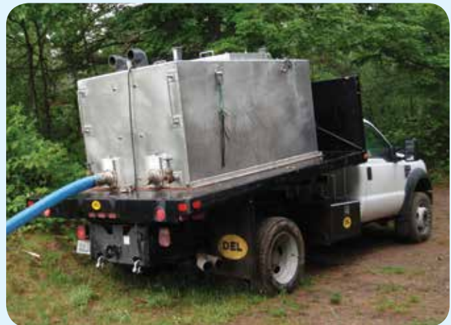
A 1-ton insulated multi-compartment truck
