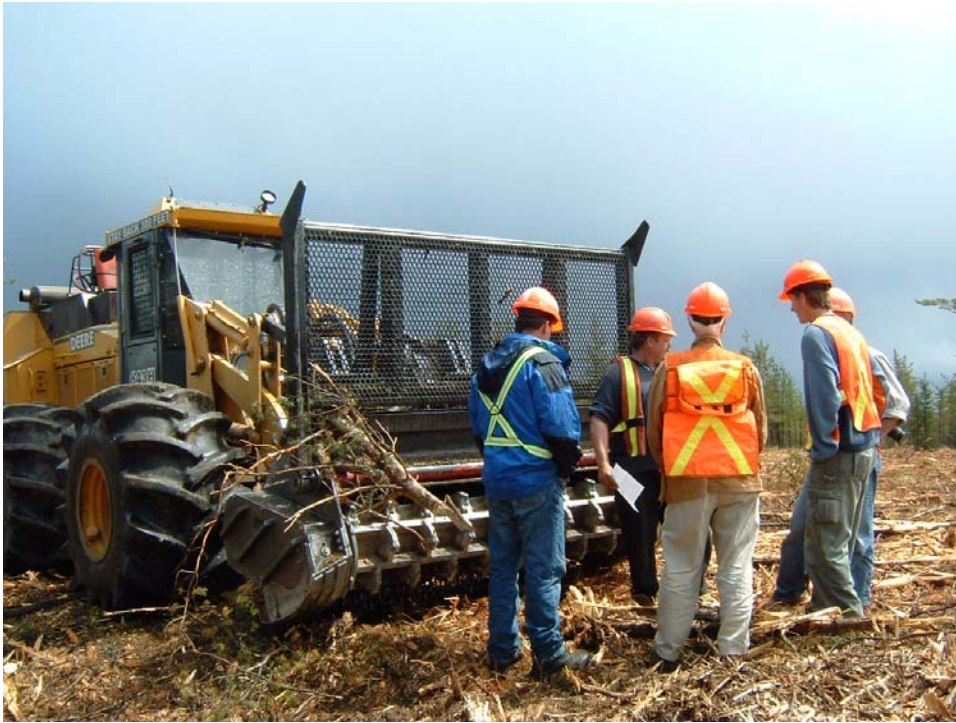
Photograph 1. Shredding equipment operated successfully among the blowdown to create an area that could be easily planted.
