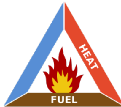
Figure 1. The Fire Triangle. Stored forage is fuel. If it heats and is exposed to oxygen, the result is a fire.
