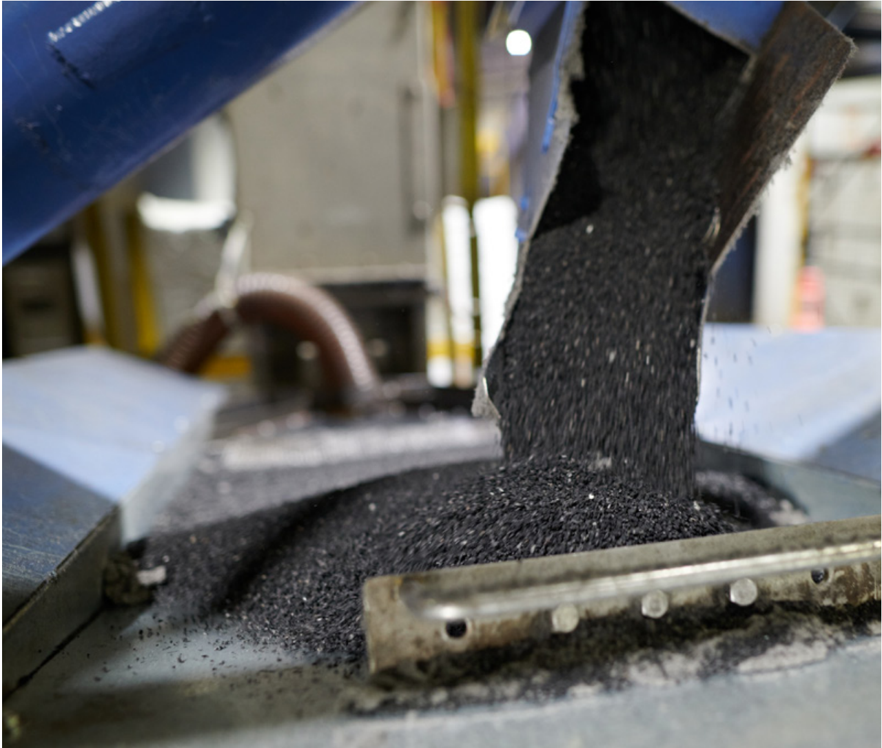
Crumb rubber created from tires at a tire recycling facility.
