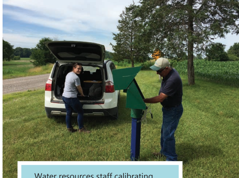
Water resources staff calibrating instrumentation that measures the water level at one of nine test wells.
