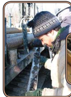
Drilling for core samples to determine the composition of the esker.
