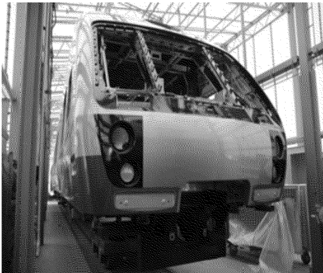
Front mask of pilot vehicle under manufacture at Nippon Sharyo plant in Japan
