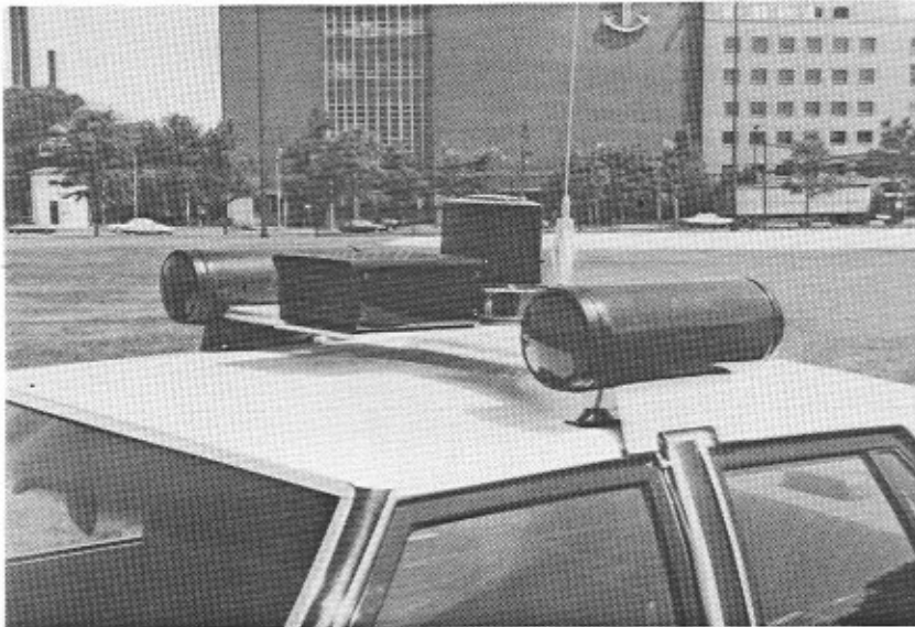
Prototype aerodynamic light-bar mounted on an OPP cruiser.
