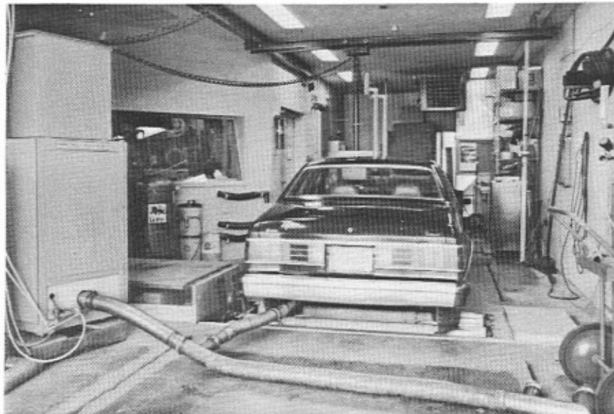
Propane-powered vehicle being tested for fuel consumption and emissions on MTC's chassis dynamometer.
