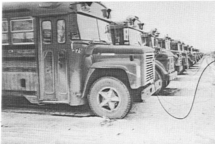
Elgin County school buses connected to the slow-fill system are filled with natural gas directly from the compressor over an interval of several hours.
