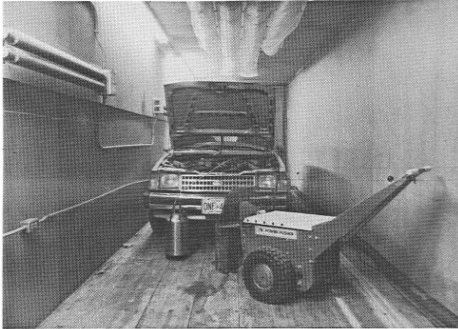
Ford Escort ready for testing in cold-start chamber.
